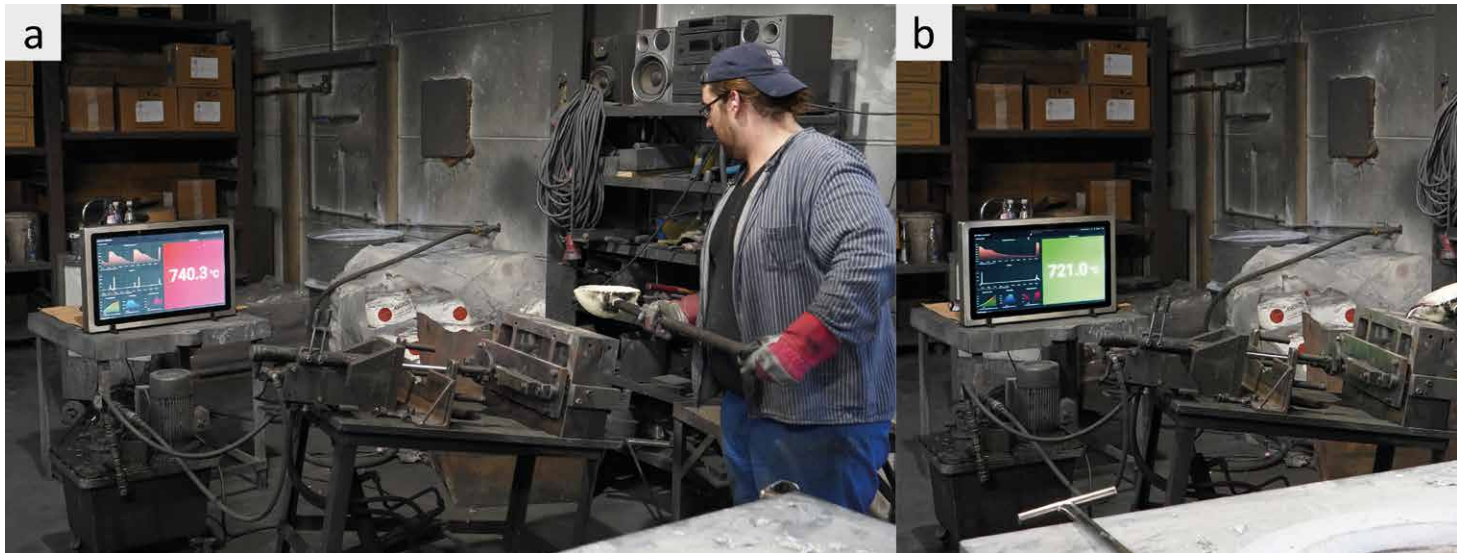
Figure 8: Application of the casting ladle 4.0 in the Hans Seifert GmbH metal foundry: a) waiting for and b) casting with color approval on a monitor at the casting station.
