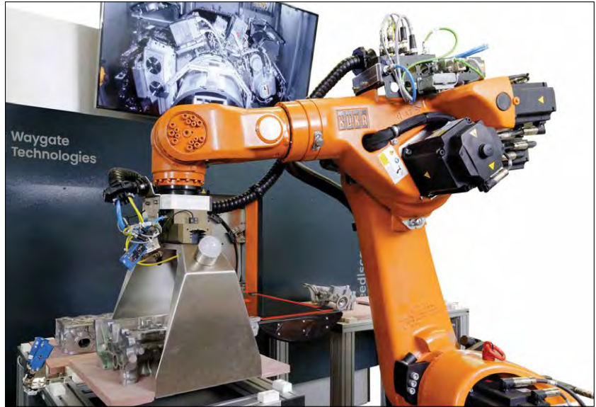
Fig. 5: Speed|scan CT64 system with robot loading for fully automated inspection.
