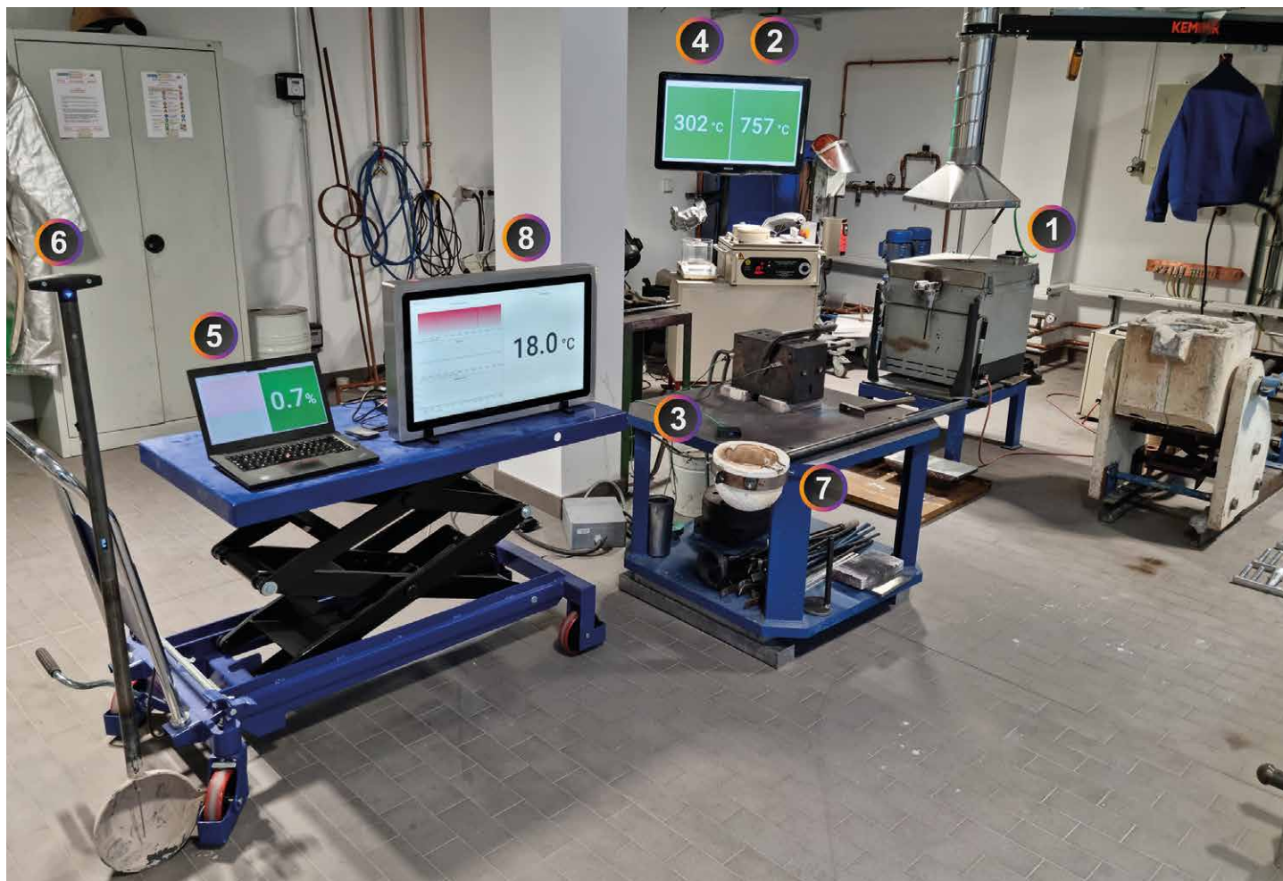
Figure 4: Selection of elements for the digitalized process monitoring in the foundry laboratory of the OVGU: 1, 2) Sensor unit for recording and real-time visualization of the melt temperature in the furnace; 3) and 4) Sensor unit for recording and real-time visualization of the mold temperature; 5) Input and visualization of further relevant parameters (here density index); 6, 7) Casting ladle 4.0 Mark I and Mark II; 8) Real-time visualization of the process parameters measured by the casting ladle 4.0.
