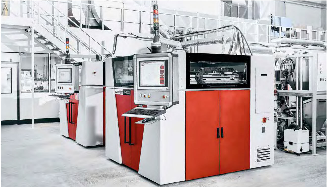
Fig. 4: voxeljet manufactures the PMMA models with the VX1000 3D printer.
